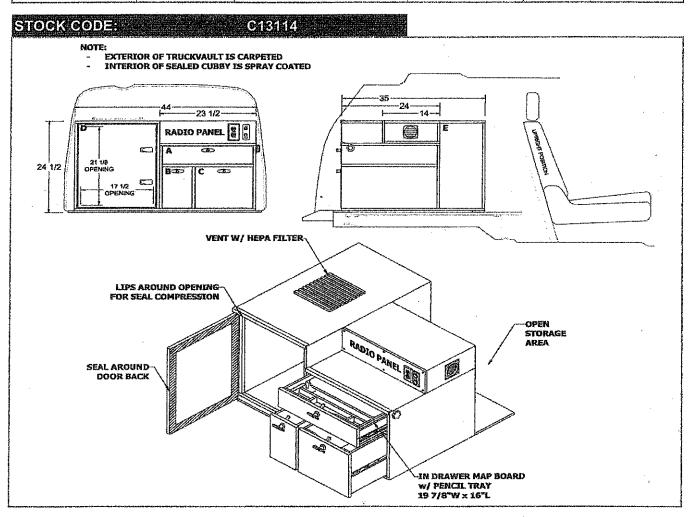
**VAULT WIDTH:** 44 **INSIDE DRAWER HEIGHT:** 4 B,C: 10 1/4 A٠ **VAULT LENGTH:** 35 **INSIDE DRAWER LENGTH:** A: 21 5/8 B.C: 22 3/4 **VAULT HEIGHT:** 24 **INSIDE DRAWER WIDTH:** 20 3/8 B; 5 1/2 C: 12 3/8 **INSIDE DRAWER DIAGONAL:** 23 C: A: 29 5/16 B: 25 1/2 **CUBBY D DIMENSIONS:** 17 1/2W x 33 1/2L x 21 1/8H OVERALL HEIGHT: 24 1/2
